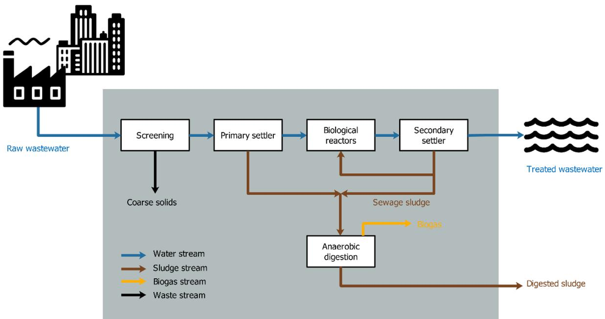
Figure 1. Simplified functional scheme of a WWTP.
