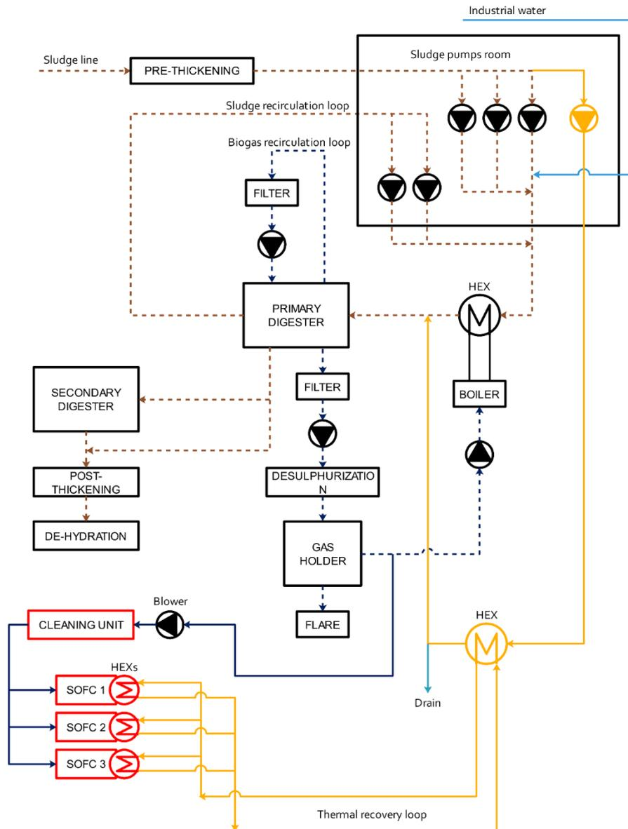
Figure 3. Biogas and sludge lines in the scenarios (2 and 3) with SOFC based CHP system.
