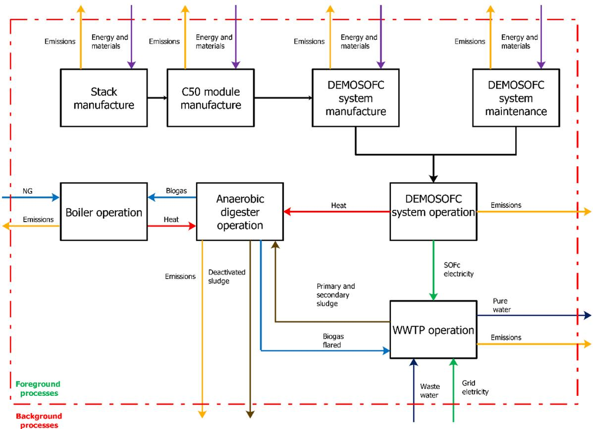
Figure 5. Boundaries of the WWTP with a SOFC based cogeneration system (scenario 2 and 3).
