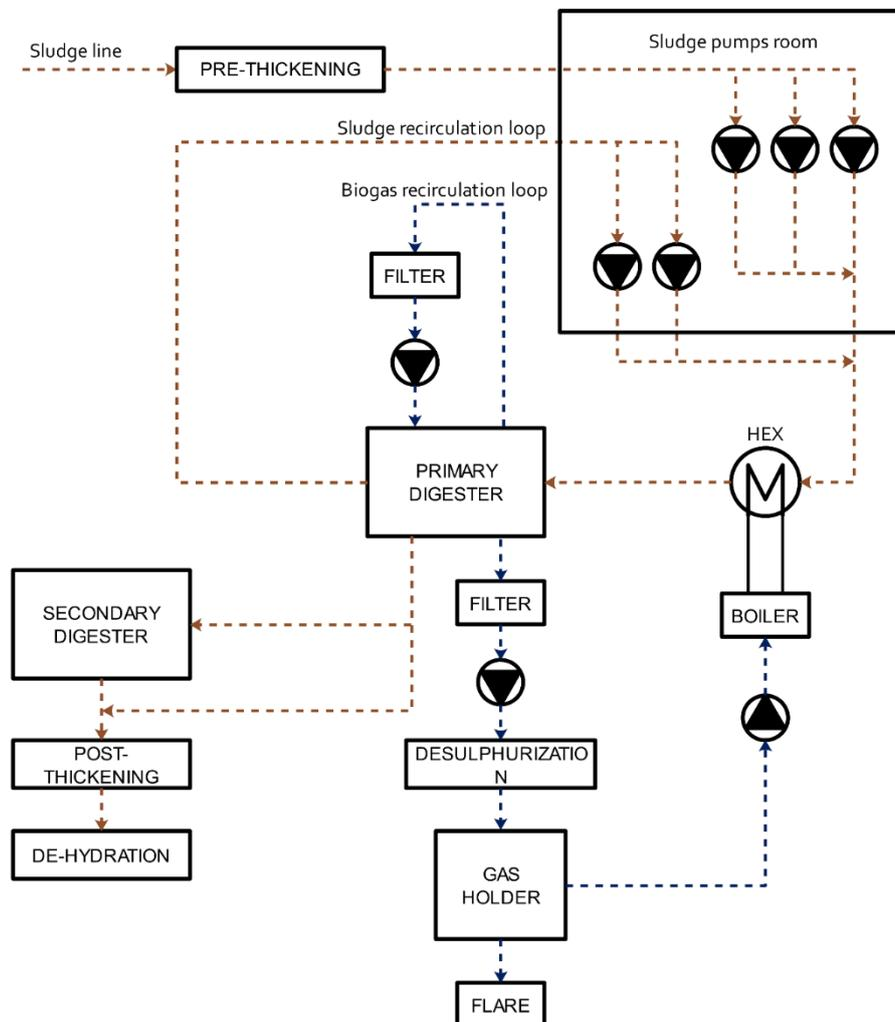
Figure 2. Scenario 1 (Reference scenario): biogas and sludge lines in the WWTP.
