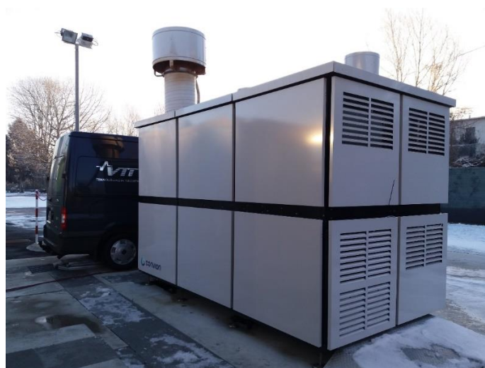
Figure 2. Setting up emission measurements. Convion C50 system in the front with VTT van with all the emission measurement equipment behind it.
